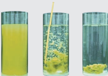
Example of a flocculation process
