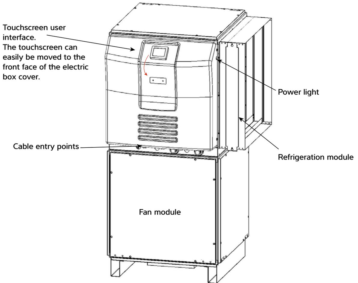
There are 3 cable glands in the electric box tray and two further knock-outs. Use the left hole for access to the power terminals. Use other available access points for the optional interface terminals.
