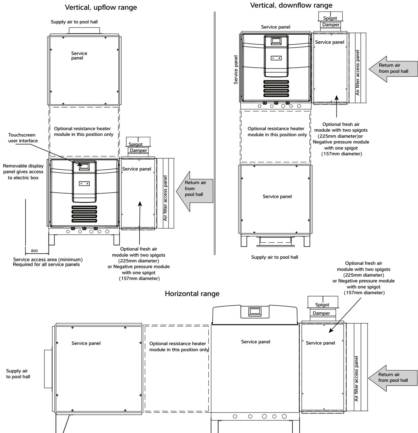
All ambient air ducting should be suitably insulated if plant room temperatures are significantly different from ambient, particularly where the plant room is at pool conditions. Spring return dampers are recommended for exhaust and fresh air ductwork in installations with sub zero ambient temperatures, in case of power failure.
