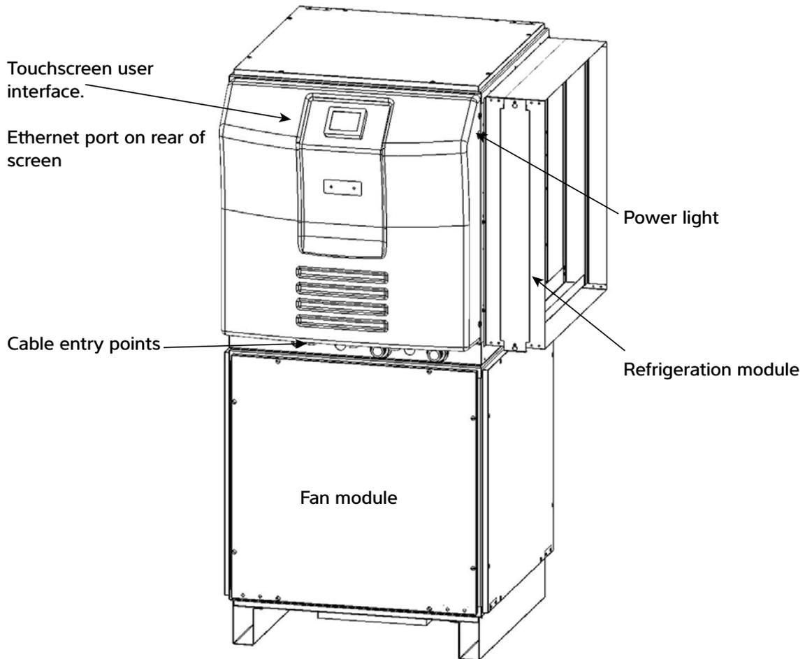
**Power light** – when illuminated red, power is connected to the Variheat.
