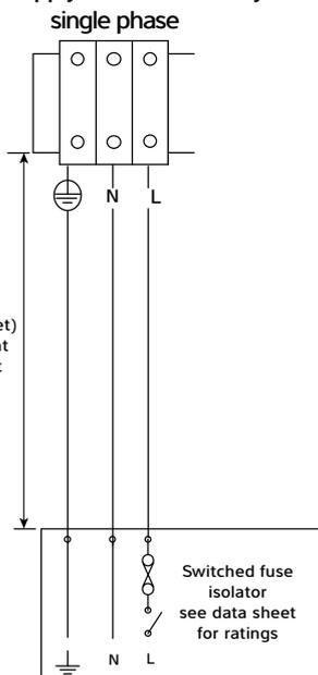
Power supply terminal block layout
