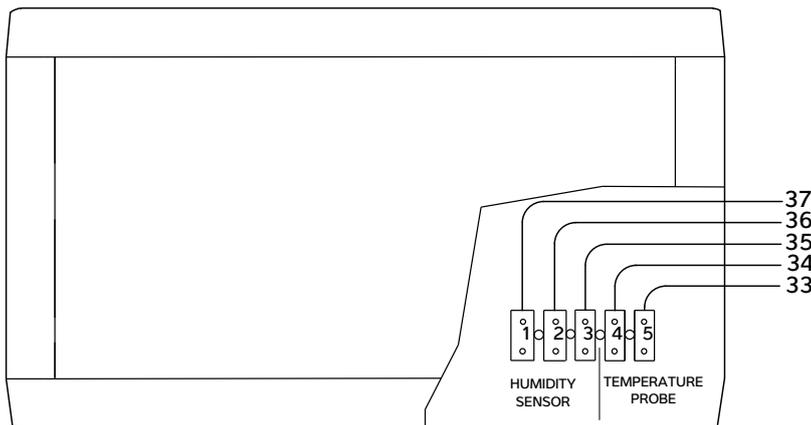
Connect terminals in sensor box to electric box terminal numbers
