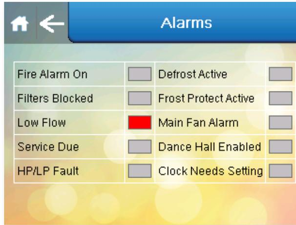
The Alarms screen displays warnings or faults with the Variheat, indicated by a red highlight. The example above indicates that there is a problem with the pool water flow rate that should be investigated.
