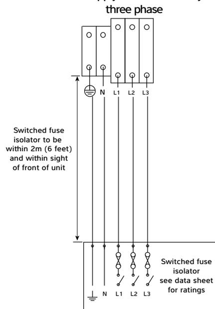
**Separate mains supply terminal blocks for resistance heater modules layout single and three phase**
