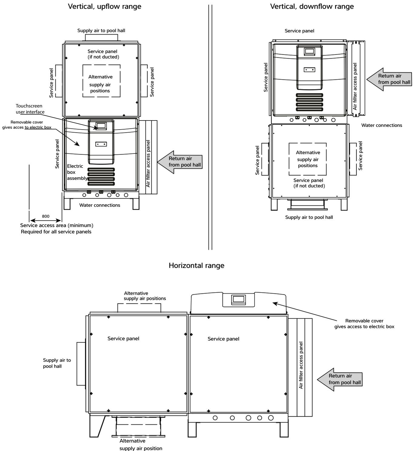
All ambient air ducting should be suitably insulated if plant room temperatures are significantly different from ambient, particularly where the plant room is at pool conditions. Spring return dampers are recommended for exhaust and fresh air ductwork in installations with sub zero ambient temperatures, in case of power failure.
