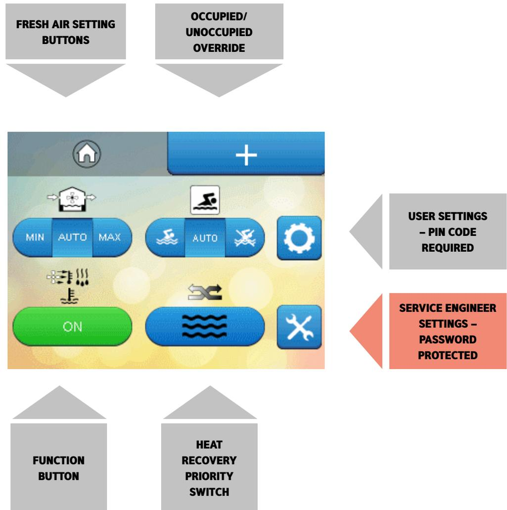
**5. Fresh air setting (where optional fresh air module is fitted)**
