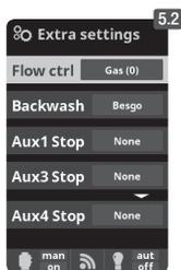
**5.2 Gas (0)** - The FL1 alarm is only activated by cell's gas sensor (external flow switch annulled).
