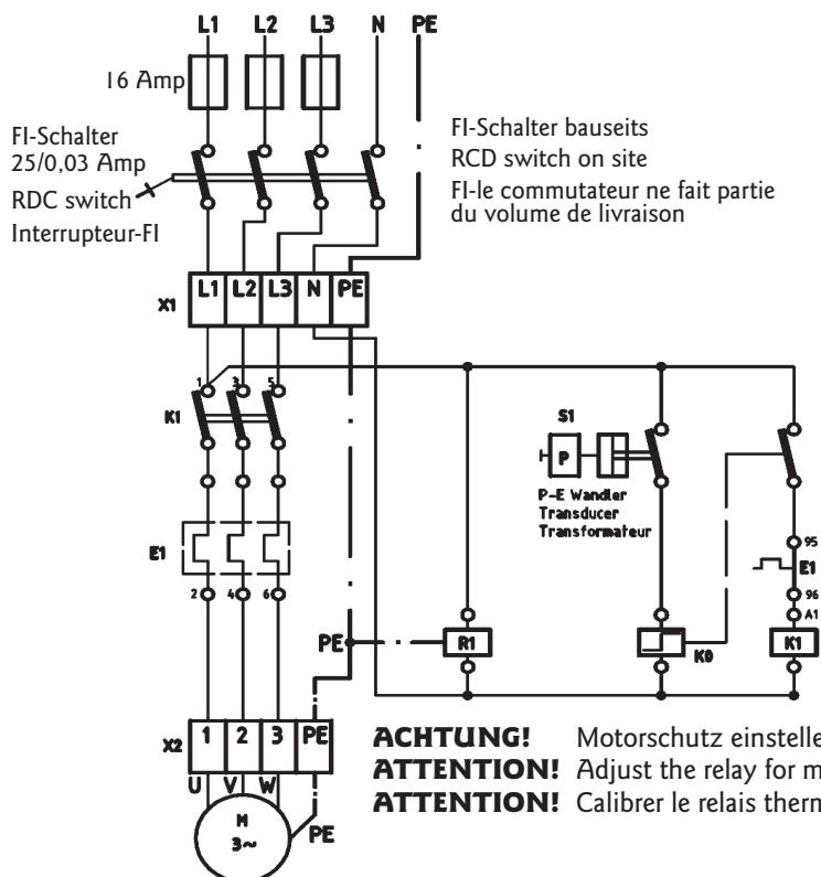
R1 Heizwiderstand / heating conductor
